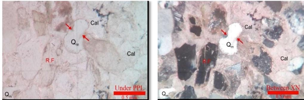
**Figure 13.** Photomicrograph showing calcite cement (Cal) corroded by monocrystalline framework grain dissolution has been quartz (Q<sub>m</sub>) of sandstone in Shwezetaw Formation
