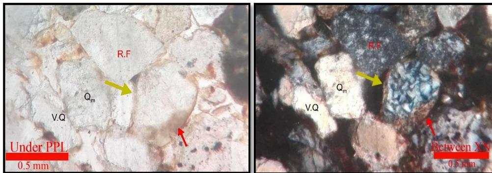
**Figure 11.** Photomicrograph pore lining clay (arrow), volcanic quartz (V.Q), monocrystalline quartz ( $Q_m$ ) of sandstone in Shwezeta Formation
